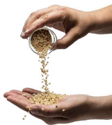
Hemp-based plastic ready to be molded
